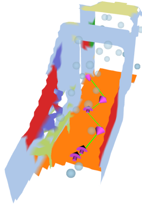
FIGURE 7.10: Visualization of the candidate viewpoints (depicted as magenta arrows) and the optimal traversal paths (green lines) in an example corridor scene. The figure also showcases the reconstructed metric-semantic mesh and the places in the DSG (blue spheres). The intensity of the place nodes indicates their utility, with darker colors indicating higher utility values.
