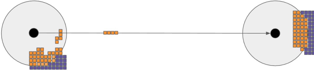
FIGURE 7.2: Visualization of the voxels of interest for two places (black dots). The colored circles represent the regions of the space that can influence the places ( i.e. , the distance to their supporting points). Unobserved voxels within the sphere and also along the ray connecting two nearby places are considered of interest (orange squares), while those outside these regions are not (purple squares). In this example, a 2-dimensional visualization is presented, voxels are considered either observed or unobserved, and only the latter are displayed.
