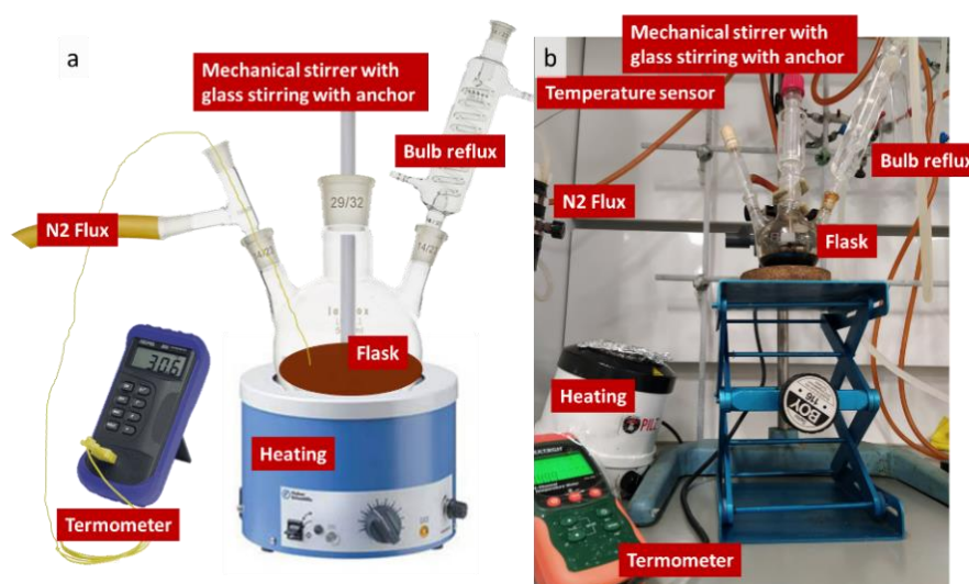
Figure 2.1. a) Schematic representation of the experimental set up used for MNPs synthesis. b) Picture of the experimental set up during the cooling fast process. In both figures, we have detailed the instrumentation used.
