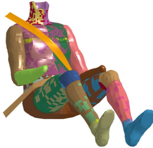
Figure 4-6: Model body parts that which mass were adjusted for the mass-scaled version.
