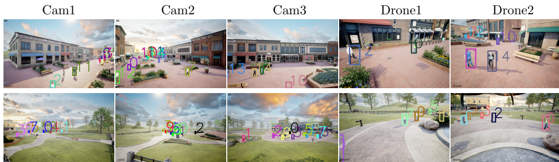
Figure 4.9: Example of images captured by the hybrid system. First row Street Busy sequence and second row Font Medium sequence. Static cameras are mainly responsible for the global understanding of the scene while mobile cameras (drones) capture pedestrian images from the desired viewpoint.
