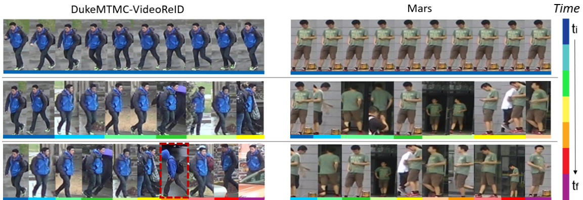
Figure 3.7: Visualization of the evolution of appearance models in the gallery. Each row corresponds to gallery samples at a certain time. The different colors represent the time stamp of the samples included in the gallery (best viewed in color).
