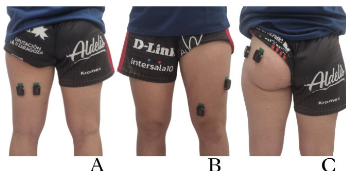
Figure 2. Location of the EMG sensors: biceps femoris and semitendinosus (A), vastus medialis and vastus lateralis (B), and gluteus maximus and gluteus medius (C).
