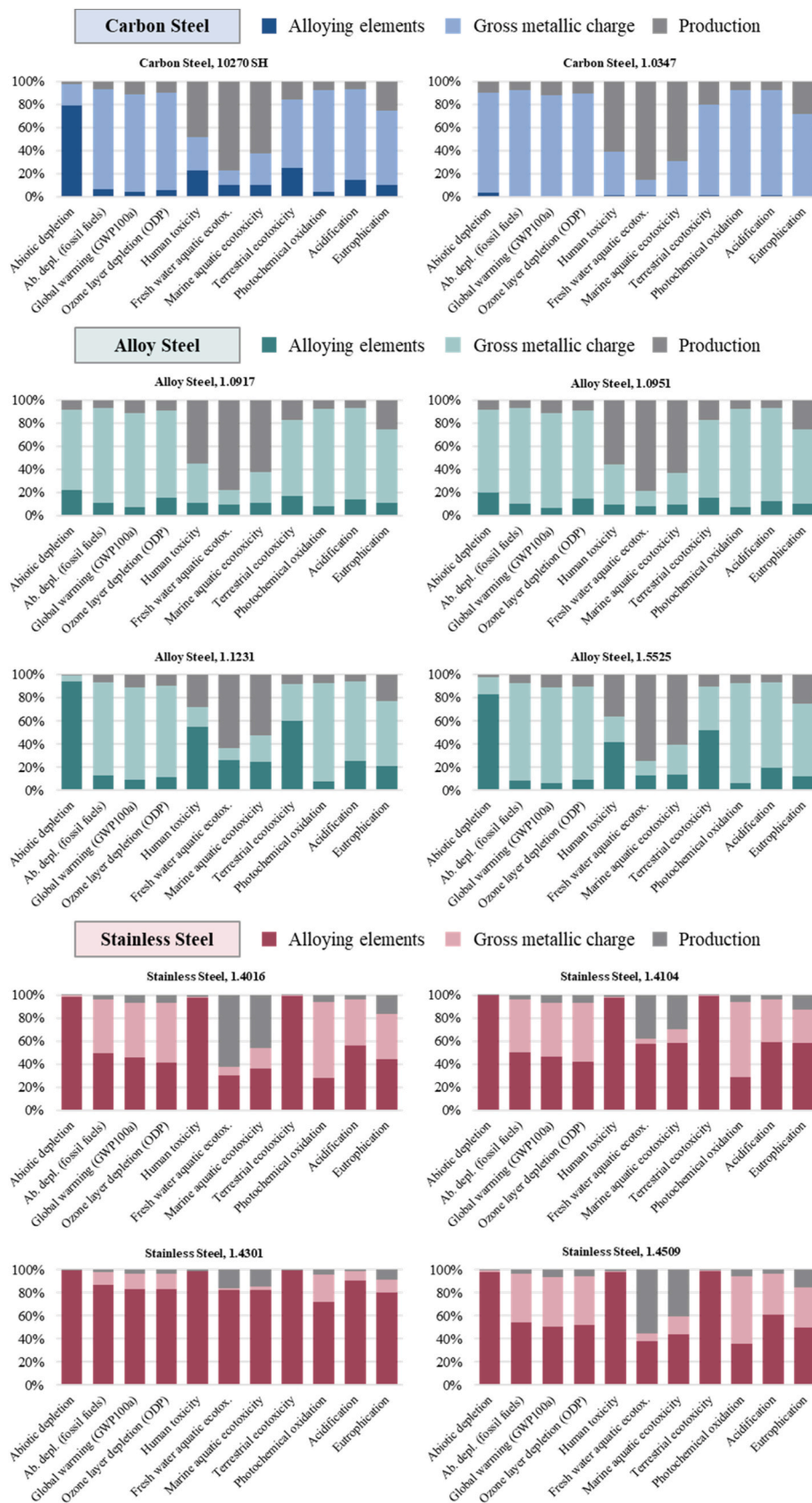
Fig. 6. Environmental impact distribution of the analysed steel grades. Alloying elements, gross metallic charge, and production process.
