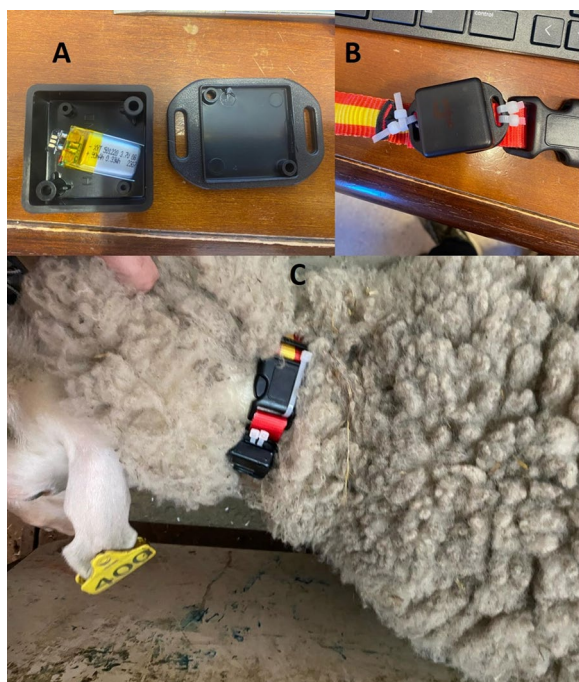
Fig. 1 Mobile Bluetooth Low Energy proximity loggers (0.9 g) (A) used in the experiment, which were protected within a plastic box (35×35×10 mm) (B) and attached to a neck collar (C)
