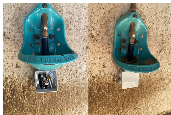
Fig. 2 Stationary Bluetooth Low Energy proximity loggers used in the experiment, which were protected within a plastic box (80×80×46 mm) that was placed under each sheep drinking trough
