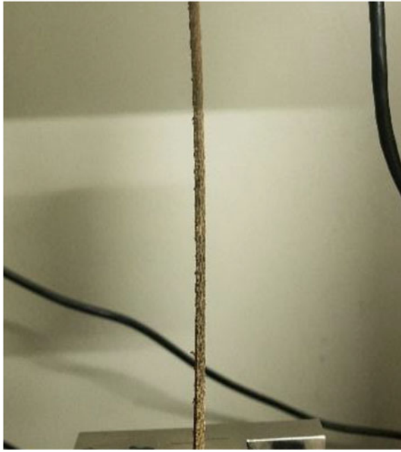
Figure 17. Set-up of the tensile test with flax fabric with 5% of humins.
