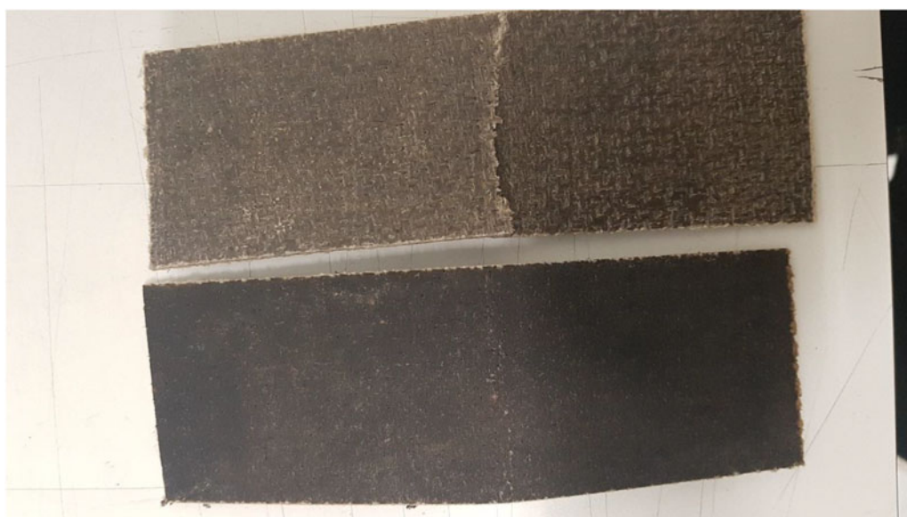
Figure 16. From top to bottom, linseed flax fabric with epoxy resin without humins and linseed flax fabric with a 15% of humins.
