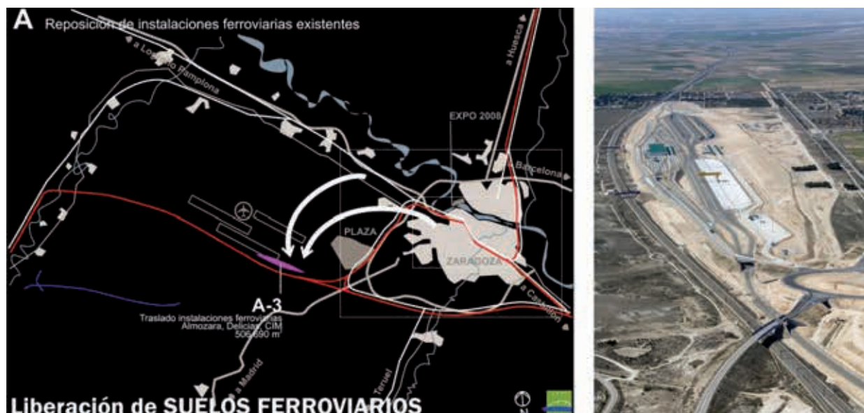
Fig 18. The relocation of the rail platform infrastructure next logistic platform PLAZA and the airport. Source: ZAV.
