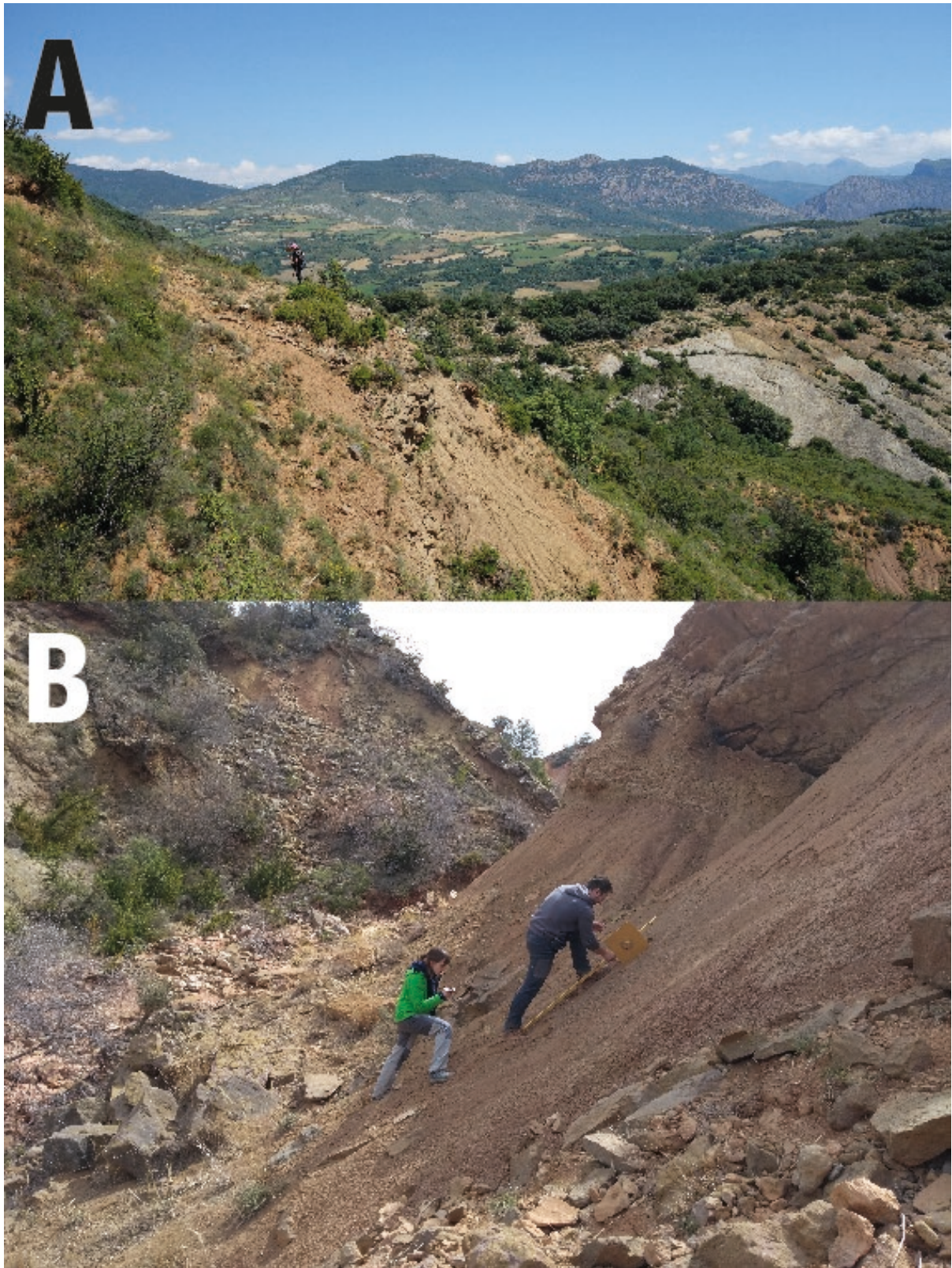
Figure 3.1. A) Measuring the Arén log with a Jacob's staff. B) Measuring a mudstone interval at the Isclés outcrop.
