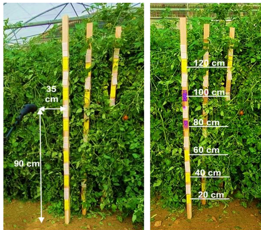
Figure 6. Water-sensitive and filter paper setting in one section in greenhouse trials.
