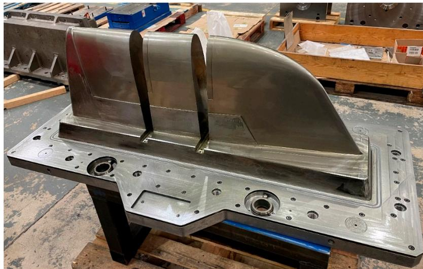
**Figure 19.** Final WAAM tooling.
