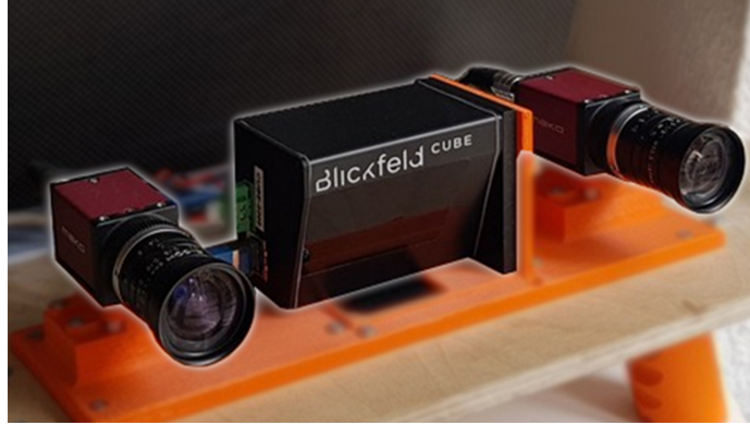
Figure 1.3: Suite of sensors onboard the LRU. Solid-State LiDAR, Inertial (S3LI).
