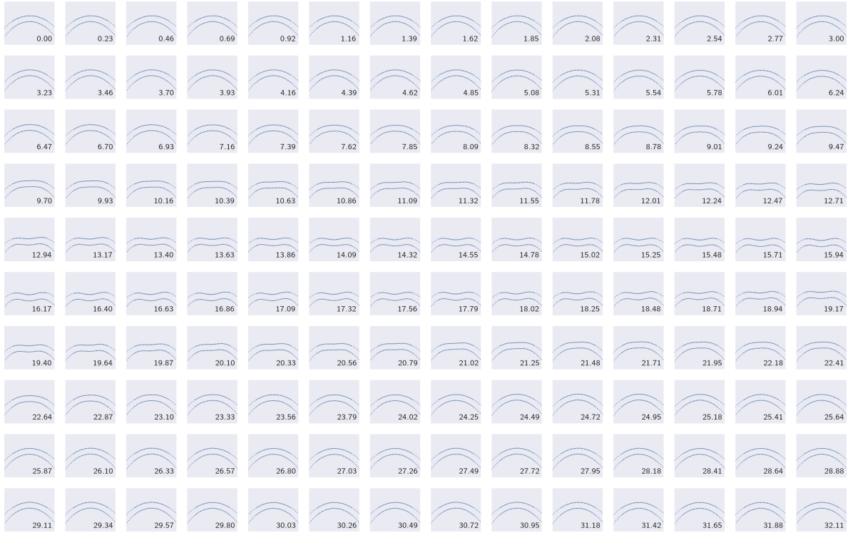
Figure 3.2: Example of FSI results. Deformation of the NT section of the cornea for different times during the simulation. The numbers reported indicate the time of the air-jet in ms.
