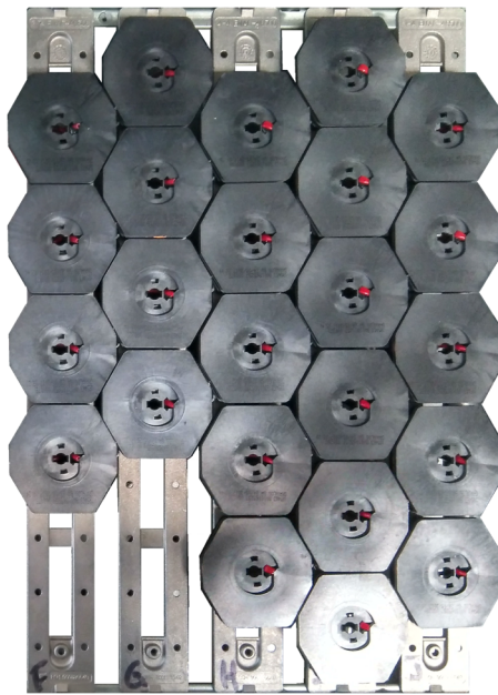
Fig. 4.3. Small inductor distribution over the cooktop surface and reference measurements.
