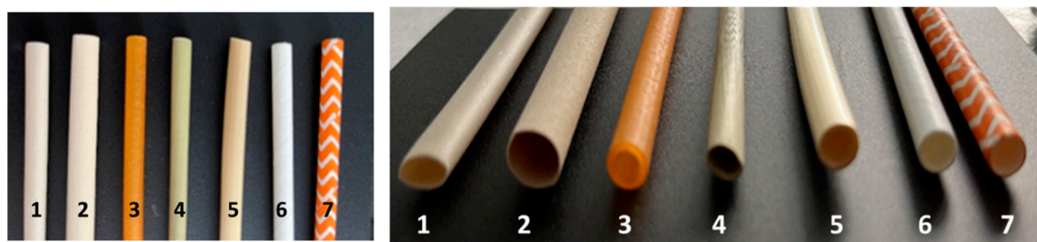
Figure 1. Images of the avocado (1), bamboo (2), rice (3), wheat (4), grass (5), paper (6), and Kraft paper (7) straws.
