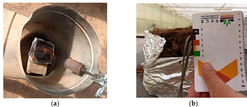
Figure 1. (a) Experimental burning setup; (b) thermocouples' arrangement at the different soil depths: 1, 2 and 3 cm.
