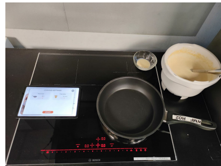
FIGURE 9. Cooking setup used during experimental validation. It consists of a PIF675DC1E induction hob y and a Balay 00570366 frying pan, an 18/10 stainless steel frying pan of 21 cm diameter.
