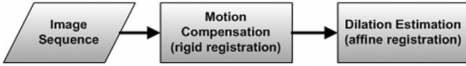
Fig. 3. Overview of the proposed two-stage method: after motion compensation is carried out by recovering a rigid motion model, the vasodilation is measured by computing the scaling factor along the normal to the artery that best matches the two analyzed frames.
