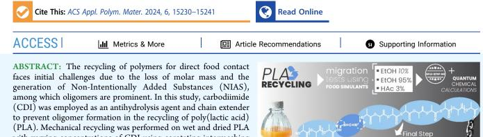
with varying concentrations of CDI using corotating intermeshing twin-screw extrusion. CDI contributed to the increase in polymer molar mass and influenced the kinetics of its nonquiescent crystallization. Moisture played a key role in this process, as CDI can react either with water molecules, preventing hydrolytic degradation, or with available sites on the PLA molecule, resulting
