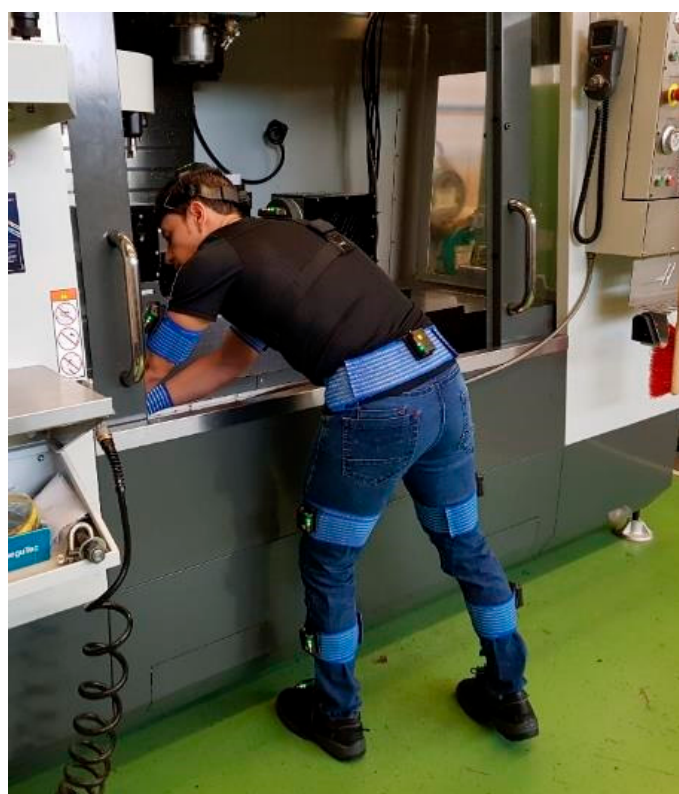
Figure 1. Motion capture in the field, placement of sensors on the worker's clothing.
