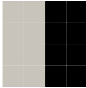
Fig. 6. Case 3. 2D mesh with the two subregions of the bed elevation.
