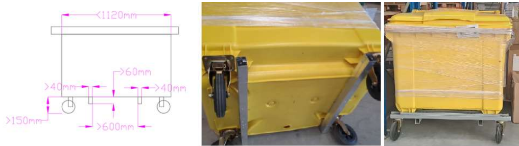
Figure 4.4.4: Modification requirement of the dust bin
