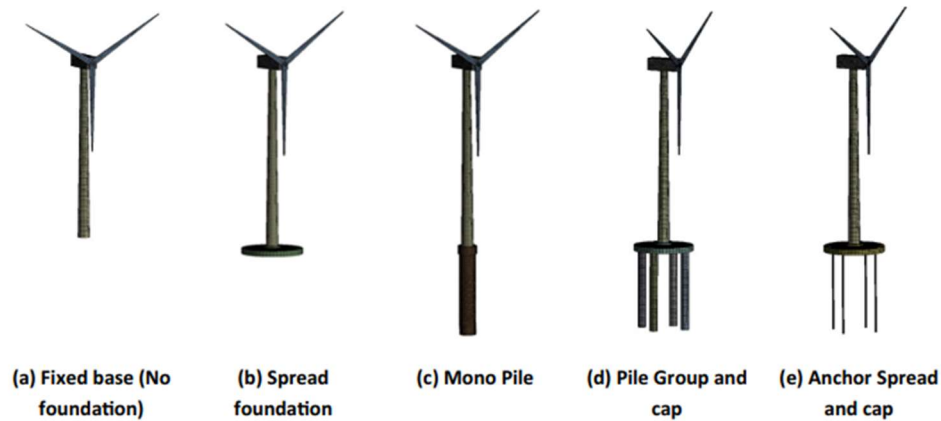
Fig. 27. Foundation types for onshore windturbines(Austin & Jerath, 2017)
