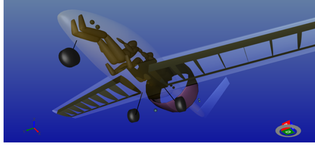
Figure 2.26 - Extended landing gear of Mindus
