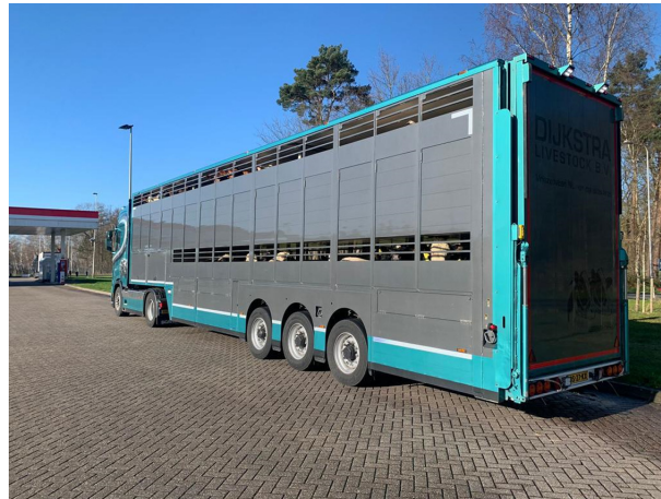
Figure 7: Two-deck cattle truck used to transport dairy heifers on long distance journeys inside and outside EU. Photo by Lars Kloster, VikingDenmark
