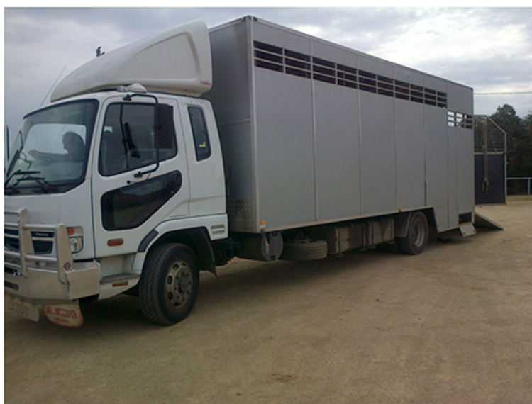
Figure 7: Commercial truck used for horses. The vehicle is passively ventilated. Source: Barbara Padalino, UNIBO
