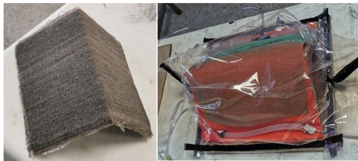
Figure 2. Resin Infusion process manufacturing for L-curved coupons of Flax Fabric and Epoxy
