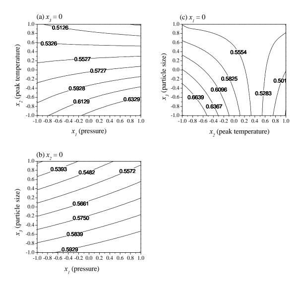
**Fig. 2**. Contour plots showing the effects on the biochar yield  $(y_{char})$  of (a) pressure and peak temperature, (b) pressure and particle size, and (c) peak temperature and particle size.
