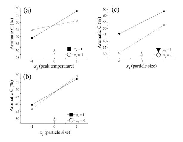
**Fig. 4**. 2-factor interaction effect plots for the percentage of aromatic C: (a) pressure and peak temperature  $(x_3 = 0)$ , (b) pressure and particle size  $(x_2 = 0)$ , and (c) peak temperature and particle size  $(x_1 = 0)$ .
