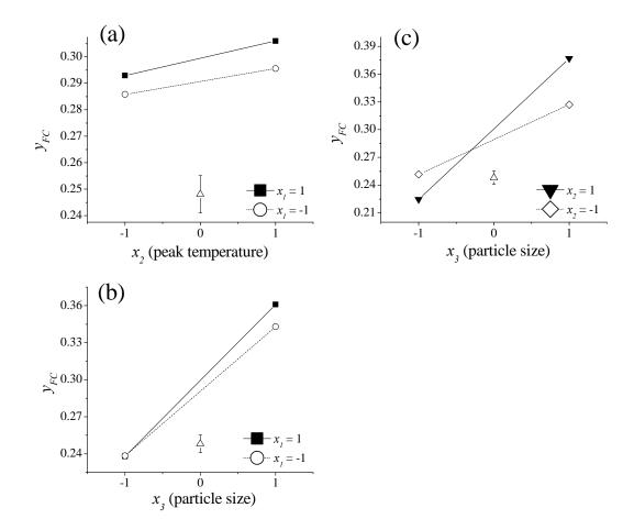
**Fig. 3**. 2-factor interaction effect plots for the fixed-carbon yield  $(y_{FC})$ : (a) pressure and peak temperature  $(x_3 = 0)$ , (b) pressure and particle size  $(x_2 = 0)$ , and (c) peak temperature and particle size  $(x_1 = 0)$ .
