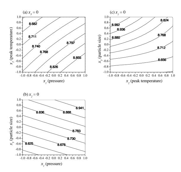
**Fig. 5**. Contour plots showing the effects on the pH of (a) pressure and peak temperature, (b) pressure and particle size, and (c) peak temperature and particle size.
