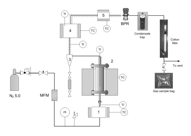
**Fig. 1**. Schematic diagram of the experimental system: (1) preheater, (2) fixed-bed pyrolysis reactor, (3) cyclone, (4) cracking reactor, and (5) hot filter.
