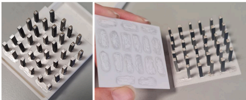
Fig. 4. Positioning the top plate according to the electrical configuration in series.
