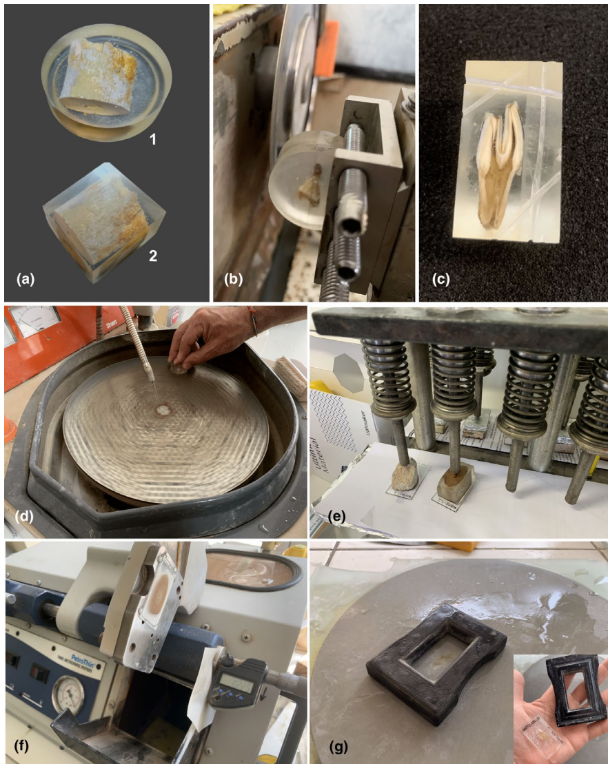
FIGURE 5 'Intermediate block elaboration' and 'Procedures for mounted block' macro-stages. Trimming process (a). A resin block is produced during embedding (a1) and the excess resin is trimmed off (a2). Sectioning of a block with an automated feed trim saw (b). The block's basal surface shows grooves made during the engraving stage (c). Polishing on an automated grinding/polishing machine (d). A press is used to keep in place the mounted blocks (e). The thin section is ground until the optimal thickness is achieved (f). Thin sections are manually polished using a holder and paper-grinding discs (g).
