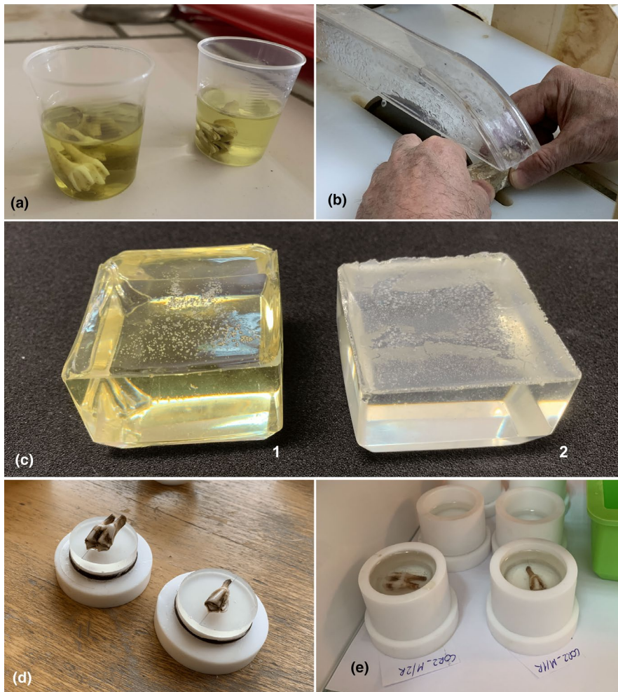
FIGURE 4 'Preliminary preparation' macro-stage. Teeth from extant specimens are dehydrated in successive alcohol solutions of 70%, 96%, and 100% (a). Extraction of a sample from a fossil specimen with a high-speed saw (b); although it is out of the scope of this work, it is worth mentioning that, when operating certain machines, protective gloves must not be used due to the risk of them getting hooked. Yellowing due to heat during resin curation (c). Resin cured at room temperature (c1). Resin cured in a refrigerator (c2). Specimens requiring a precise section are mounted on cured resin bases with the section plane marked on them (d). Specimens are placed in moulds in which the resin is poured until it covers them (e).
