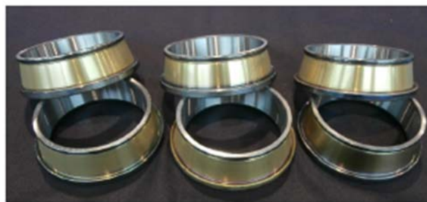
Figure 13. Bearing samples D4 coating + B polish post-processing.
