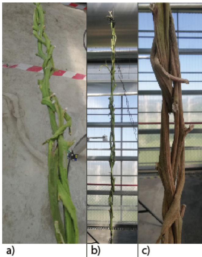
Fig. 12. Braiding and resistance test of tomato stems: a) Braiding process; b) fresh braided stems carrying weight; and c) detail of braided dry stems.
