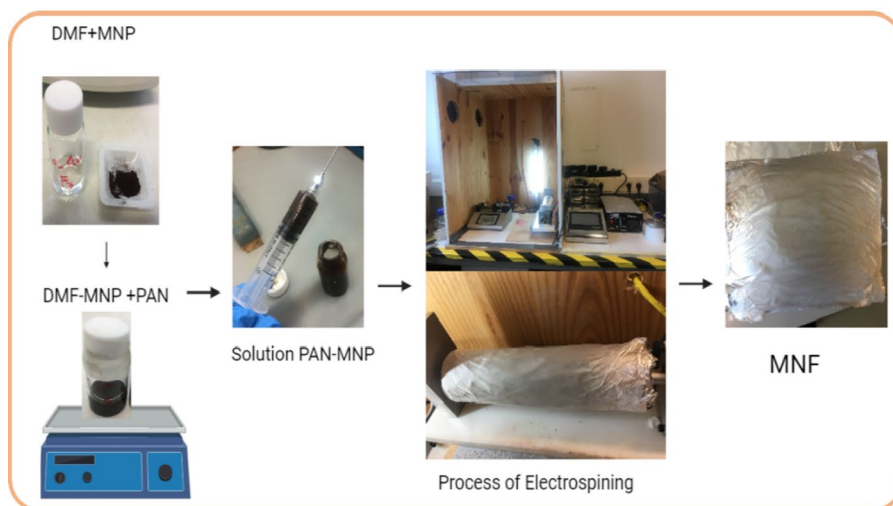
Fig. 1 Organic matrix (polyacrylonitrile, PAN) with inorganic particles (magnetite, MNP) hybrid membrane's (MNFs) elaboration using electrospinning processing. MNP were dispersed in a suitable solvent (dimethylformamide, DMF), the dispersion was heated and mixed with PAN powder. After overnight stirring at room temperature, the solution was electrospun and the obtained fibers collected in an aluminum foil
