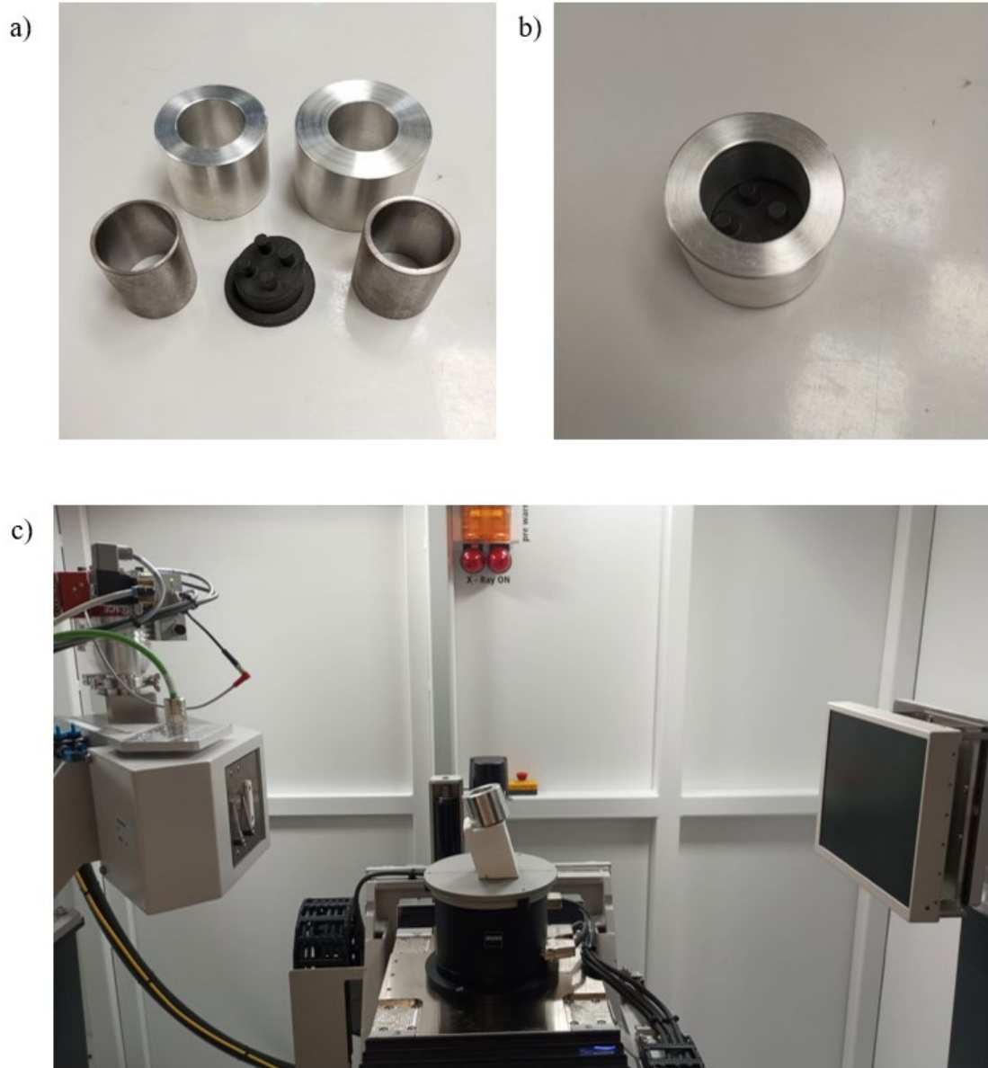
Figure 4.17. Details of the manufactured test object. a) Individual parts (hollow cylinders and base). b) Assembly (Al 20 mm). c) Test object positioned on the XCT device.
