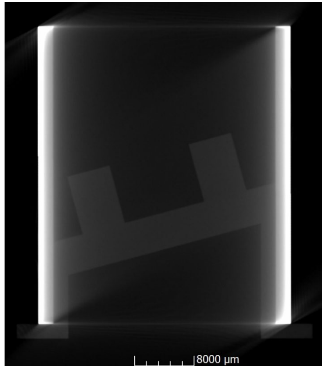
Figure 2.3. 2D slice of a simulated XCT evaluation of a metal-polymer assembly
