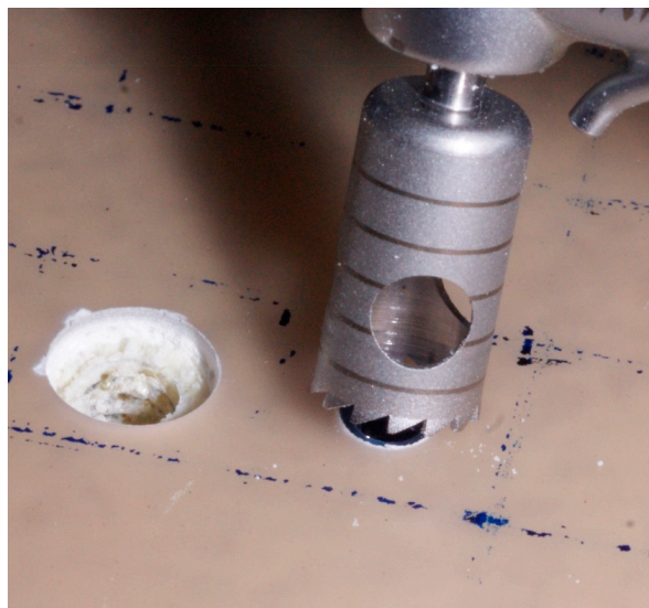
Figure 2. The trephine used for bone defect simulation.
