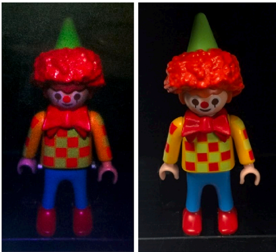
Fig. 12. Comparison of the wavelength multiplexed hologram (left) and the real object (right).
