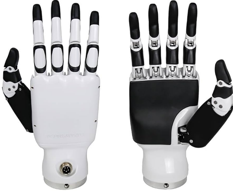
Figure 1.1: Modern humanoid robotic hand showcasing advanced design for grasping and manipulation.
