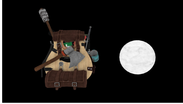
(c) G-Buffer texture that stores the albedo reflectances of fragments in our renderer.
