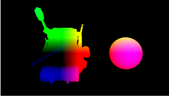
(a) G-Buffer texture that stores the world-space position of fragments in our renderer.
