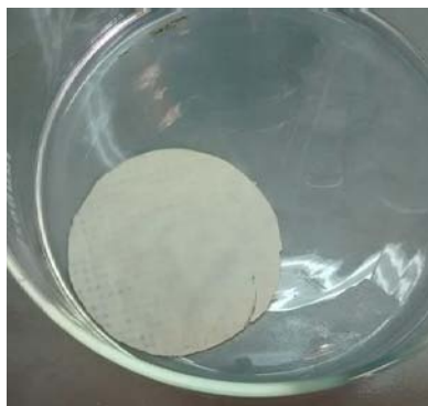
Figure 36 Final experimental set-up of big scale ZIF-8 synthesis on electrospun PBI membrane
