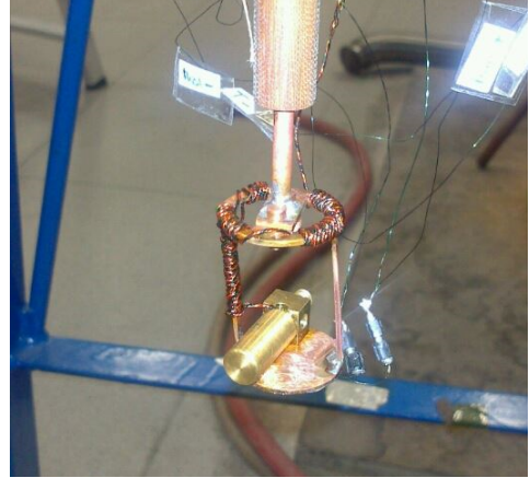
Fig.10: Quasiadiabatic calorimeter developed in the Low temperature laboratory.
