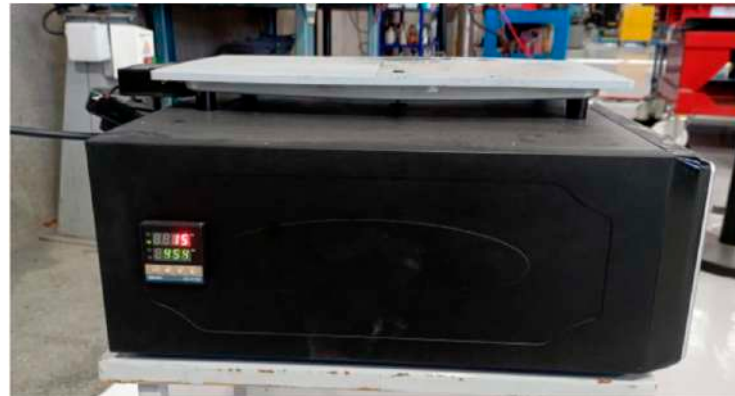
Figure 4. Images of the electric griddle instrumented with a PID-controlled thermostat, used for the heating tests.
