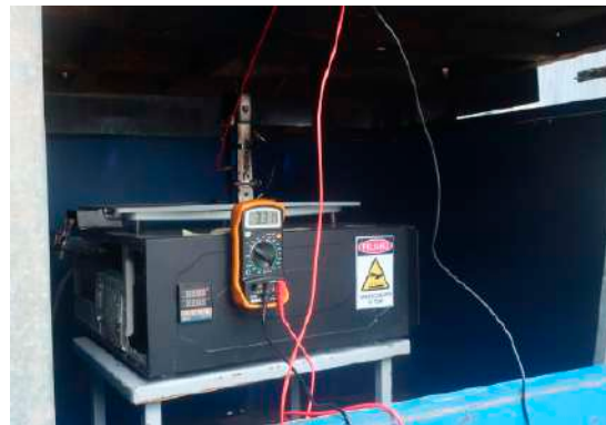
Figure 44. Image of the cells with an SoC of 50%, placed with a tool in a vertical arrangement and connected in parallel on the electric griddle, before the starting the heating test.
