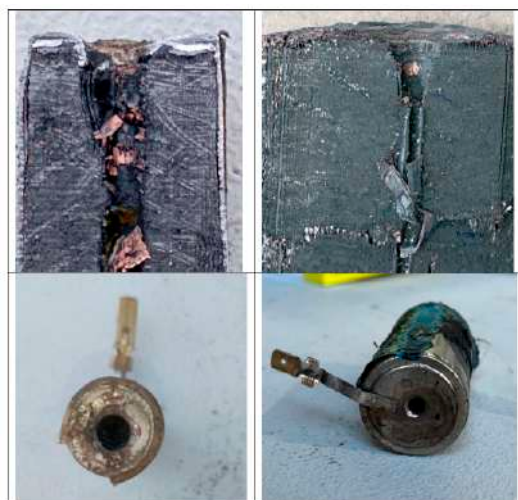
Figure 28. Qualitative comparison of the damage in the NMC cell ( left ) with the damage in the LFP cell (cell C) ( right ), tested by mechanical abuse by perforation in the direction of the longitudinal axis of the cell.
