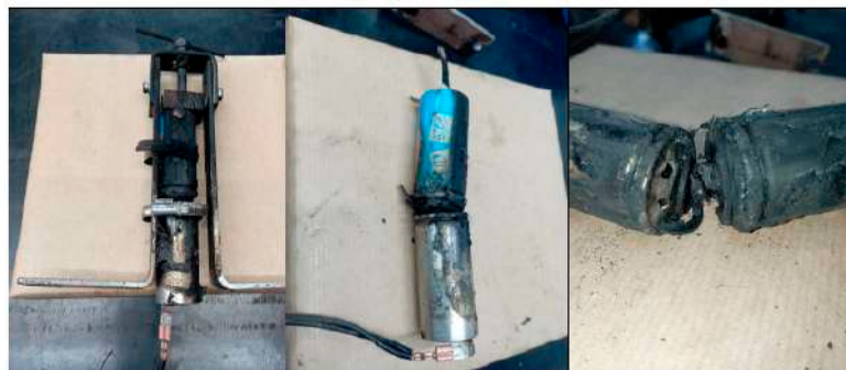
Figure 45. The first image shows the two cells with the tooling used to prevent the cells from moving during the test. The second and third images show the state of the cells after test 5.
