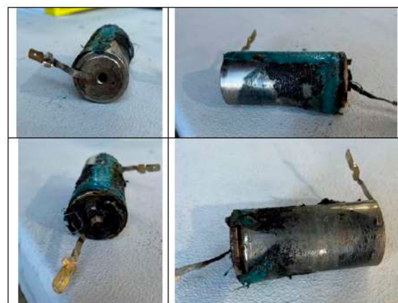
Figure 15. The state of cell C after the test, where the perforation it has undergone is clearly visible.
