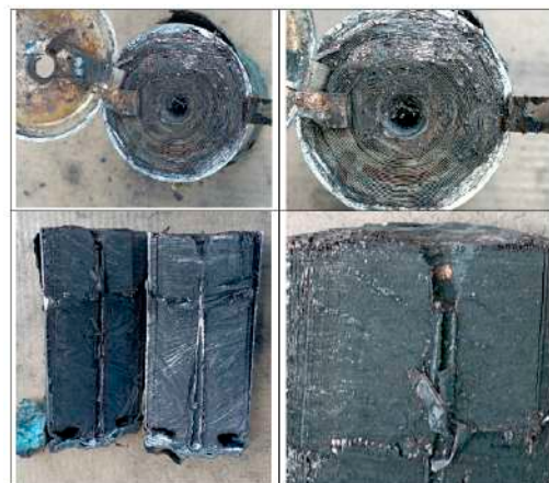
Figure 17. Image of the damage in cell C tested for mechanical abuse by perforation in the direction of the longitudinal axis of the cell.
