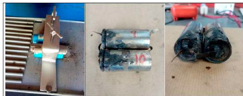
Figure 40. The first image shows the two cells before the test with the tooling used to prevent the cells from moving during the test. The second and third images show the condition of the cells after test 3.
