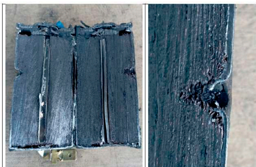
Figure 8. Image of damage to A cell tested for mechanical abuse by perforation in the direction perpendicular to the longitudinal axis of the cell.
