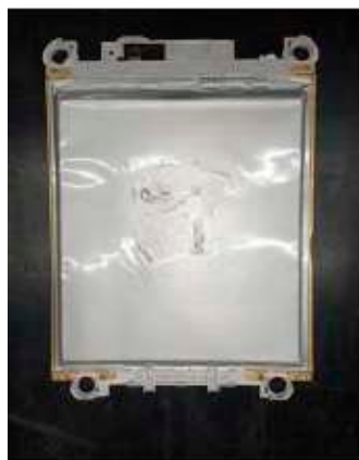
Figure 32. Image of the pouch cell in its original state to be used in the overcharge tests.
