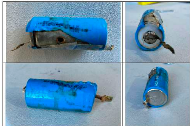
Figure 10. Images of the state of cell D after the test are shown, where the perforation it has undergone can be clearly seen.
