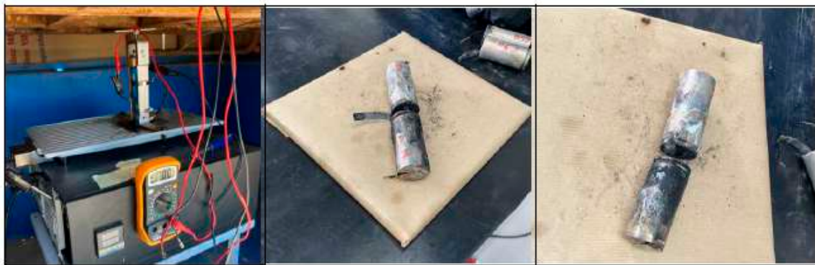
Figure 42. The first image shows the two cells on the electric griddle with the tooling used to prevent the cells from moving during the test. The second and third images show the condition of the cells after test 4.
