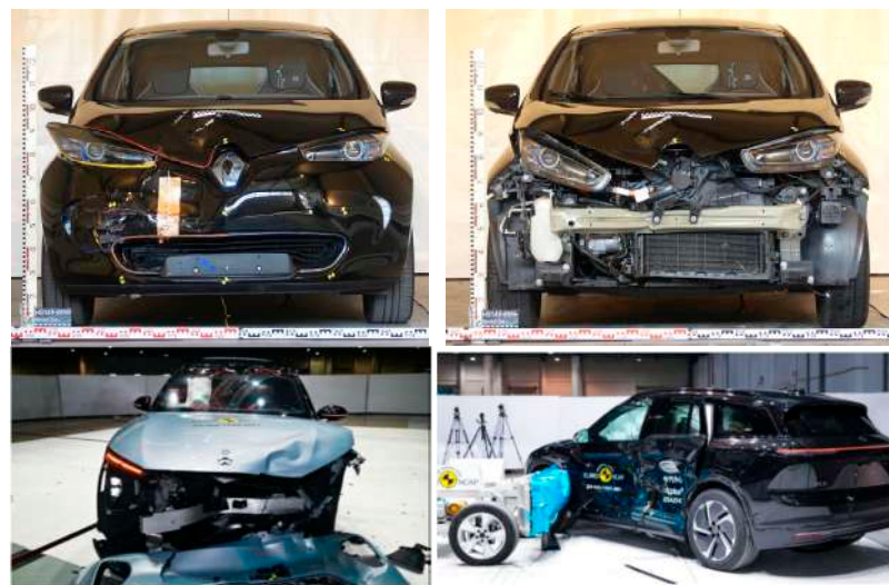
Figure 2. Images of various deformed electric vehicles in a crash test. Source: Renault Zoe (at the top) [70] and NIO EL6 (at the bottom) [71].
