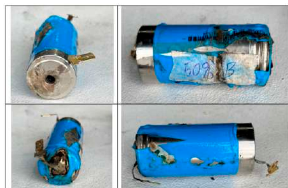
Figure 19. Image of the damage in cell B after the test; the perforation is clearly visible.
