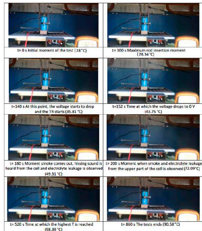
Figure 22. Images of the main events experienced by cell B (SoC 50%) during the mechanical abuse test (perforation in the direction of the longitudinal axis of the cell).
