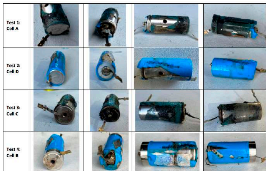
Figure 23. Qualitative comparison of the final state of the tested cells (analyzing their exterior).
