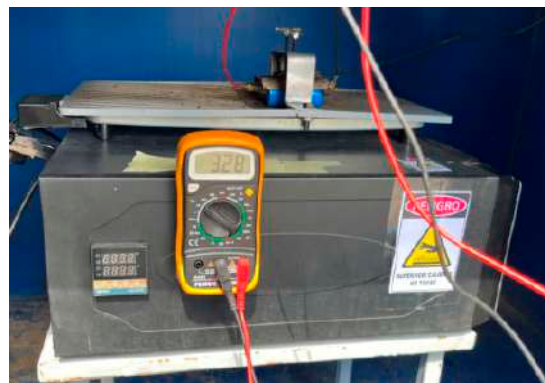
Figure 47. Image of the cells with an SoC of 50%, placed with a tool in a horizontal arrangement and connected in parallel on the electric griddle before the starting the heating test.
