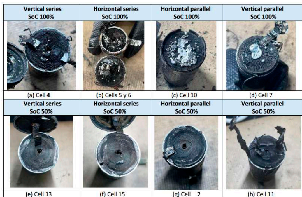
Figure 54. Final state of the cells after thermal abuse tests by heating, after removal of the top cover.
