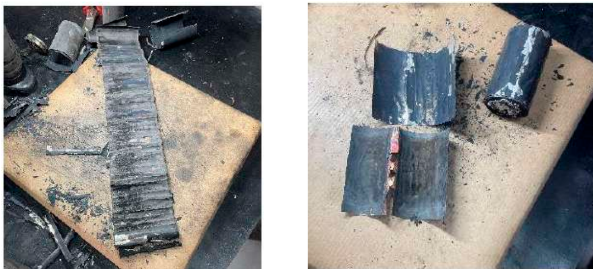
Figure 55. Final state of tested cell 7 (Test 4: vertical arrangement parallel connection SoC 100%) (left) and final estate of tested cell 10 (Test 3: horizontal arrangement parallel connection SoC 100%) (right).
