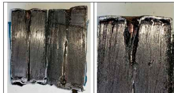
Figure 21. Image of the damage in cell B tested (SoC 50%) for mechanical abuse by perforation in the direction of the longitudinal axis of the cell.
