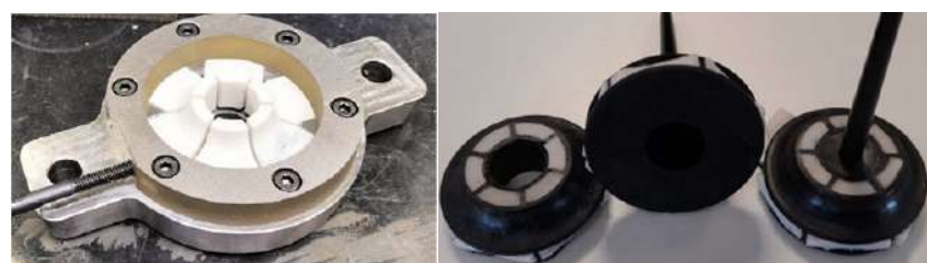
Figure 14. Salt removable inserts and injected samples.
