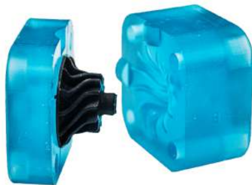
Figure 2. Example of a dissolvable resin mold (xMOLD).
