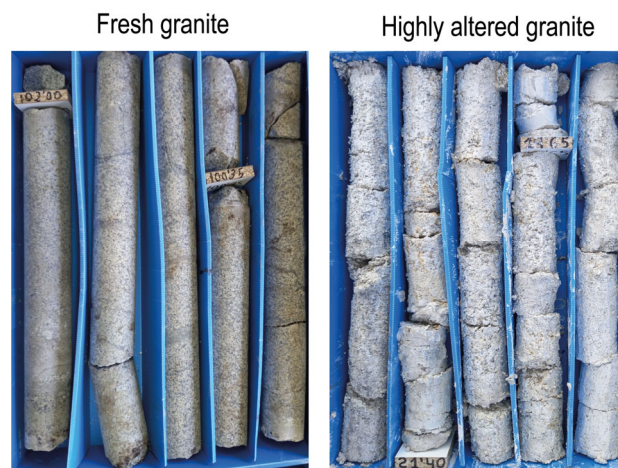
Figure 2. Boreholes of fresh and highly altered granites.
