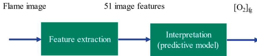
Fig. 3. Method for the processing of flame images.
