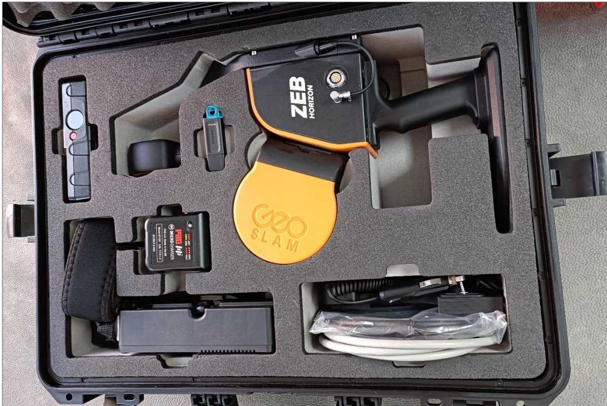
Figure 2.12. The GeoSLAM ZEB-Horizon full system, including HMLS unit (above-right) and ZEB-Horizon real-time datalogger (below-left).
