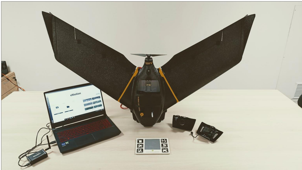
Figure 2.10. The eBee Classic full system: UAV unit (center), eMotion software and ground USB modem (left), Airinov reference target (center), and the two optical sensors (right).
