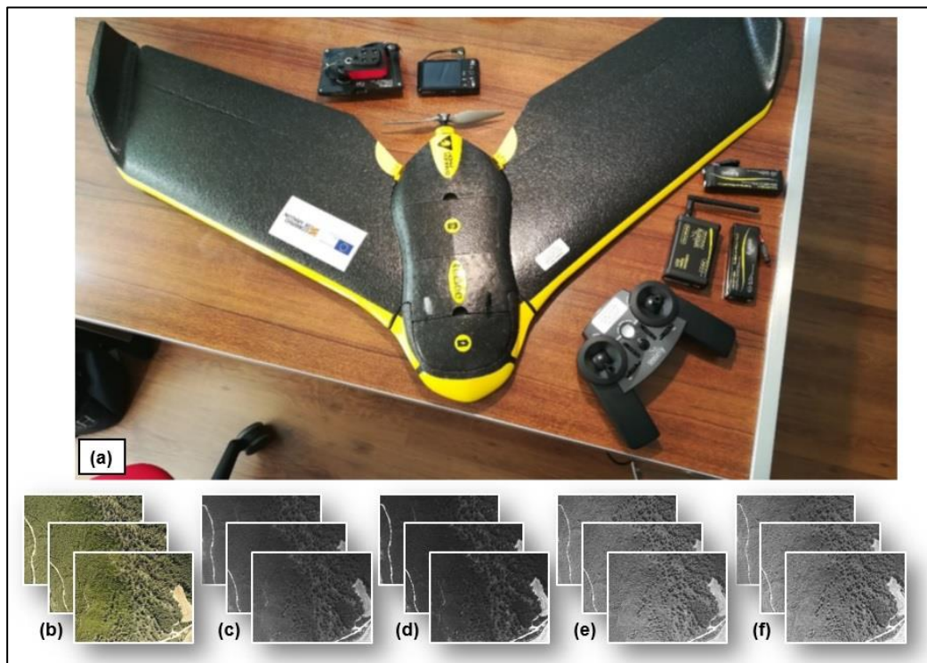
Figure 2. Above: (a) Main materials used in the study: SenseFly eBee Classic UAV unit with SONY WX camera and Parrot Sequoia multispectral sensor. Below: Examples of the same single image captured by the UAV in different spectral bands: (b) RGB; (c) Green band; (d) Red band; (e) Red-edge band; and (f) Near infrared band.
