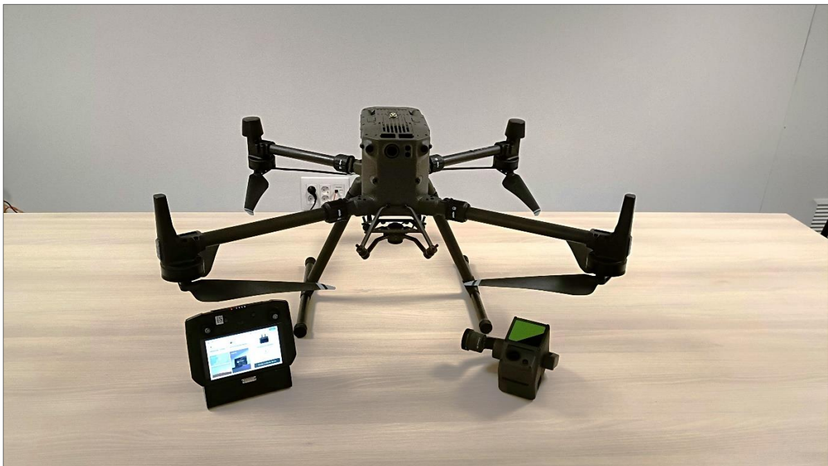
Figure 2.11. The UAV-LiDAR full system: DJI Matrice 300 RTK UAV unit (center), controller (left), and DJI Zenmuse L1 LiDAR sensor (right).
