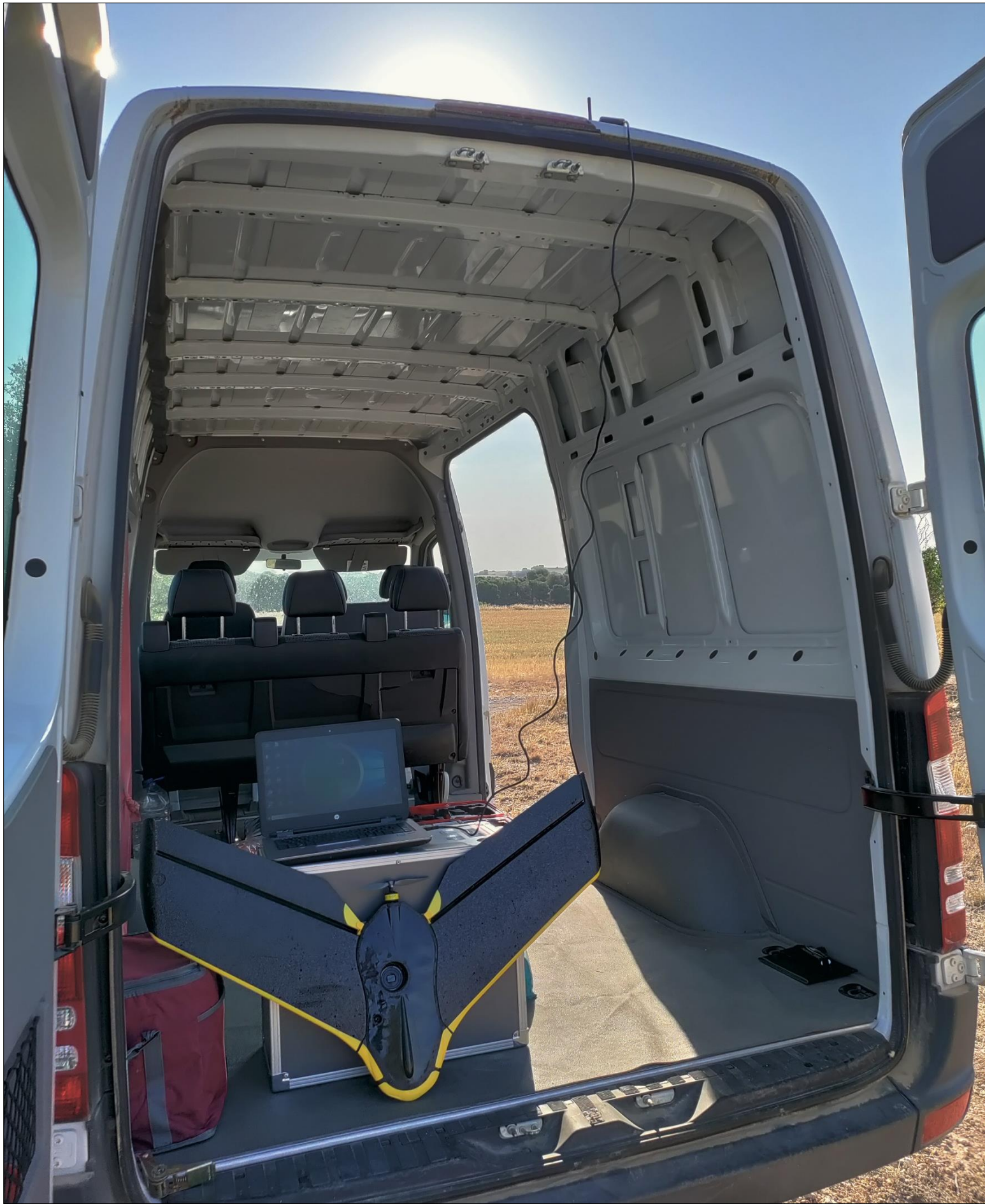
The eBee Classic UAV system. Photograph by Raúl Hoffrén.
