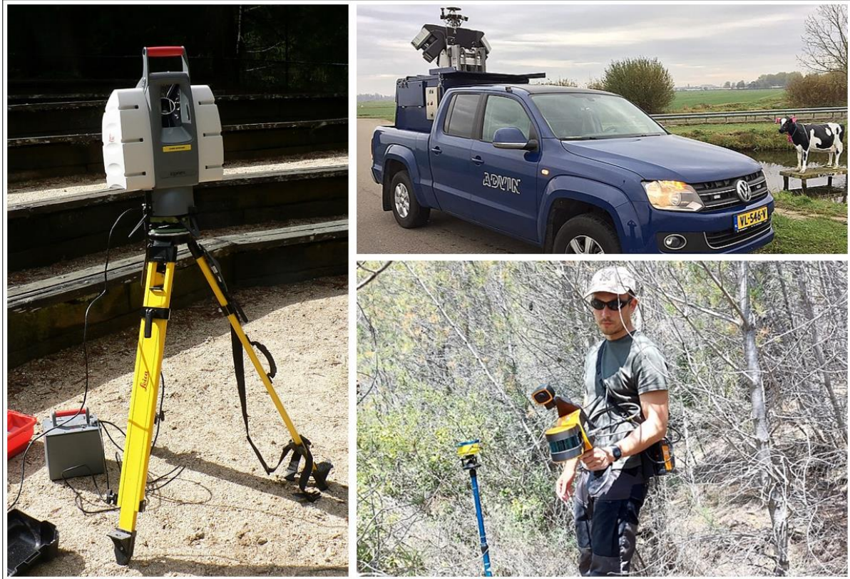
Figure 1.3. The three main platforms of ground-based laser scanner systems in forestry: TLS (left), MLS (above-right), and HMLS (below-right).
