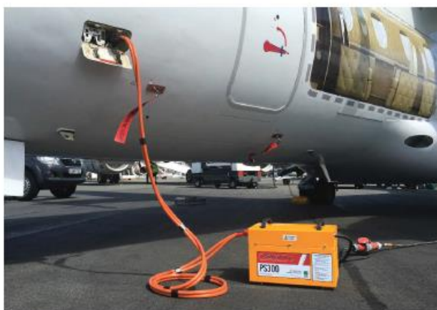
PS300: In operation on a Dornier 328
