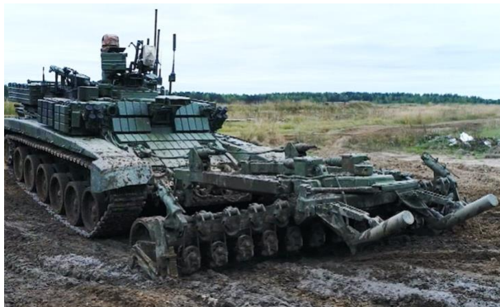
Figura 10. Prokhod equipado con rodillos. Fuente: https://rtd.rt.com/series/combat-approved-series/prokhod-armour-plated-minesweeping-robot/
