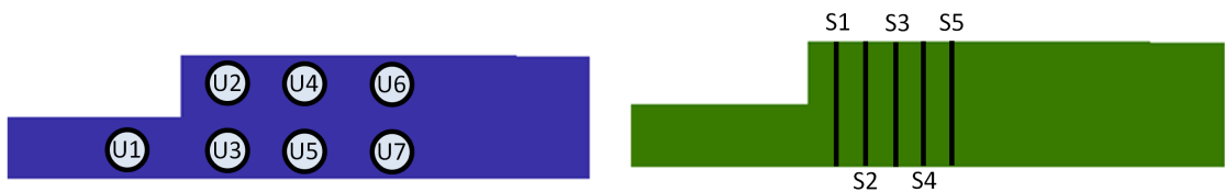
Figure 9.18: Plan view of the experimental flume. Locations of the probes (left) and the cross sections (right)
