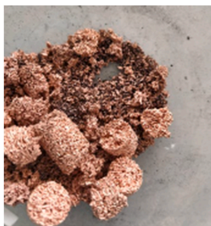
Fig. 7. Carbon deposition after an experiment with a CuO bed (experiment 4.1).
